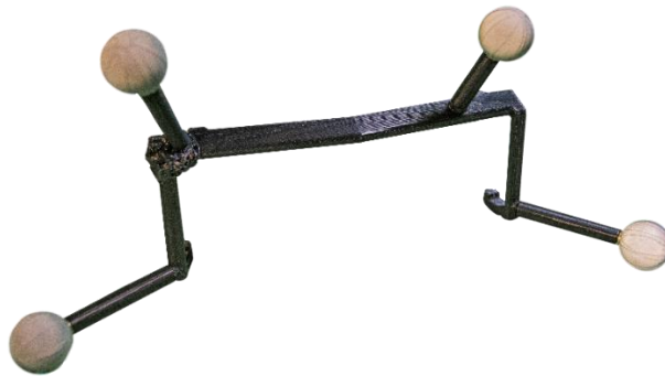
3D Printed, Mountable Retroreflective Passive Markers for Tracking Head Pose
